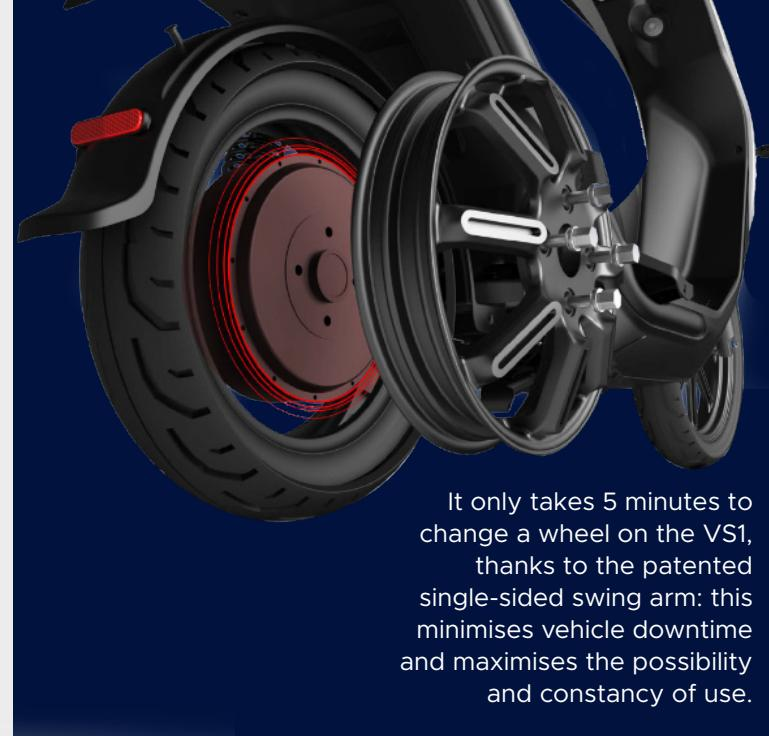
It only takes 5 minutes to change a wheel on the VS1, thanks to the patented single-sided swing arm: this minimises vehicle downtime and maximises the possibility and constancy of use.
